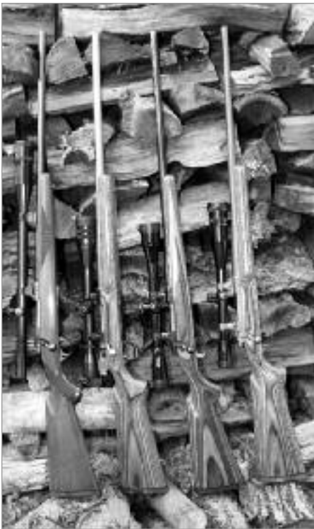
The four Ruger .220 Swift rifles owned by Munnell in order as described in the text. From left: M 77 V, M 77 Mk II VZ, M 77 VZ and M 77 Mk II VT. The only external difference between the second and fourth rifle is the metal coloring. The third rifle does not exist, according to the Sturm, Ruger & Co. factory records.
